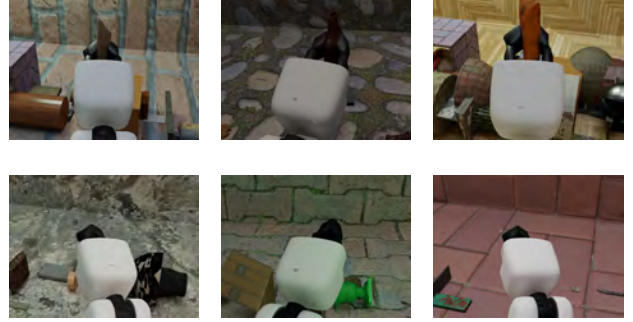
Fig. 1: Examples from the proposed dataset. The top row shows examples with an object within the gripper while the lower row corresponds to no object. Each example corresponds to a different batch.
