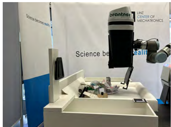
Fig. 4. Container with opened bottom. The container will be placed on the fixture after closing the bottom.
