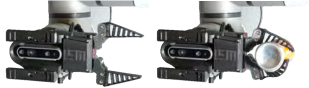
Fig. 7. Elastic fingers with fin ray design in opened and closed configuration. (The LED lights still need to be installed next to the Realsense camera.)
