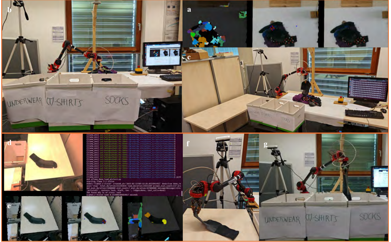
Fig. 2: Procedure of the experiment. A single piece of garment is identified by the grasp prediction algorithm (a), the robot then picks up the garment (b) and places it on the inspection table (c). The VLM identifies the type of garment and its color (d). The grasp prediction algorithm is then run again to identify the optimal grasp position (e). The garment is then picked up (f) and placed in the dedicated container (g). Unrecognized or not categorized are discarded at the back of the table for further manual inspection.
