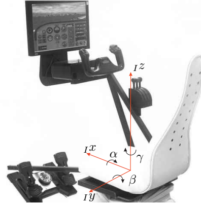
Fig. 1: Motion simulator mounted on the parallel platform
