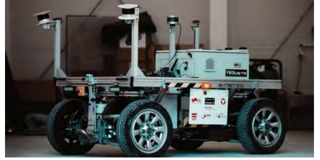
Fig. 2. The experimental robot setup equipped with two 32-layer Hesai LiDARs.
