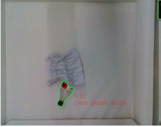
Fig. 10. Output of the YoloV8 model: visible contour (shown in green) and label (with confidence) of the object.
