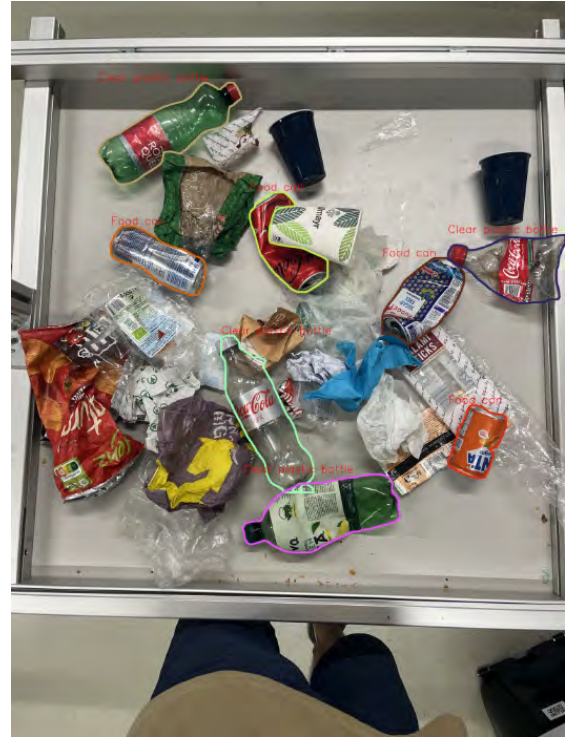
Fig. 9. Validation of the segmentation: Result of the YOLOv8 model with the same picture as in the training.
