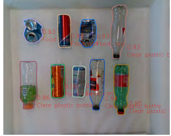
Fig. 13. Test objects with their classes according to the YoloV8 model.
