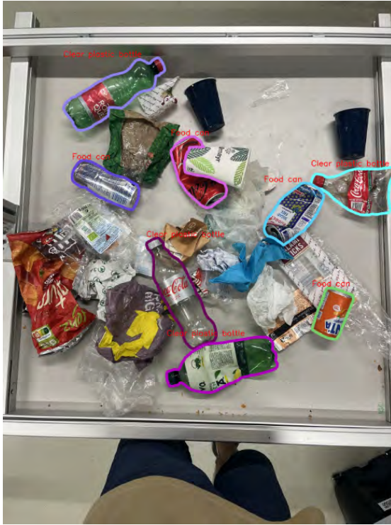
Fig. 8. Validation of the segmentation: The training data labeled with the offline tool based on SAM.
