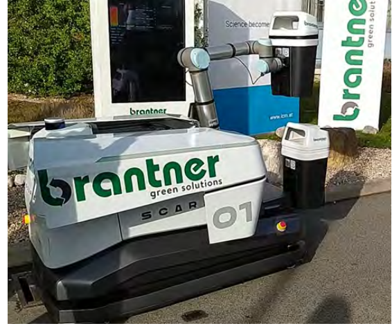
Fig. 1. SCARAB during operation while changing the container.
