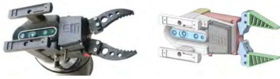
Fig. 6. Different designs of the gripper: Left with rigid fingers, right with fin ray design. In the right figure, the Gimatic gripper is shown in red and blue and the capacitor box is under the lid with the LCM logo.
